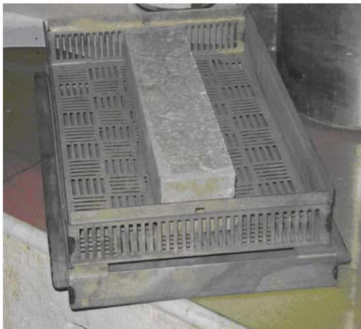
Figure 15: Specimen of concrete for pavements, stored in a curing chamber and then subjected to temperatures between 350 and 450°C in an oven
