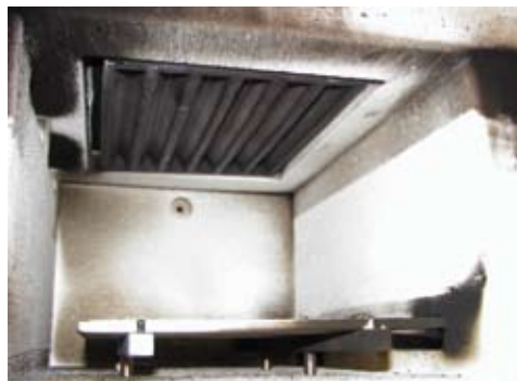
(c) Inside of the oven with the infrared heaters at the top
