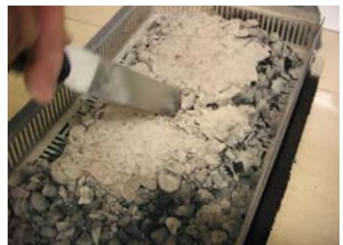
(f) Once the test is completed the bituminous mixture loses completely its cohesion and can be easily broken off
