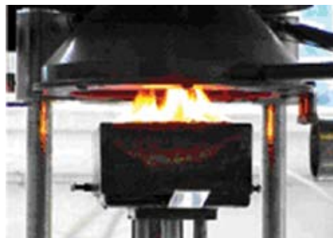
Figure 13: Ignition of a specimen of bituminous mixture in the cone calorimeter test
