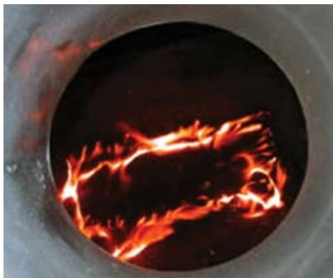
Figure 8: Specimen of bituminous mixture during its ignition (Cergy – Pontoise University)
