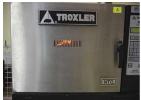
(d) Ignition of the bituminous mixture during the test
